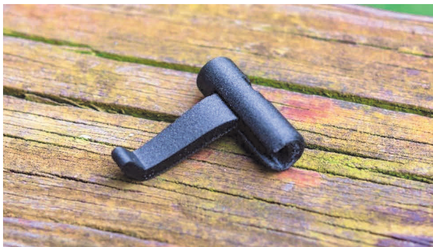
Figure 15. Test fitting the lever in the cam.
