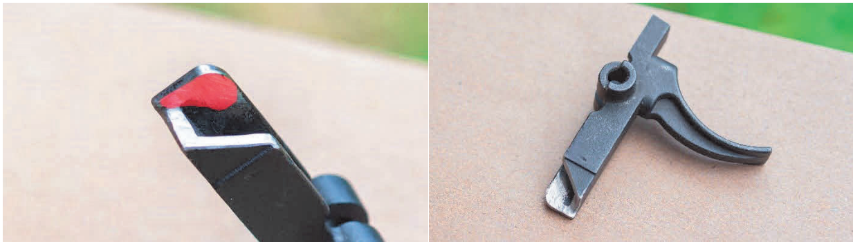
Figure 12 and 13. Final adjustment grind. Completed trigger.
