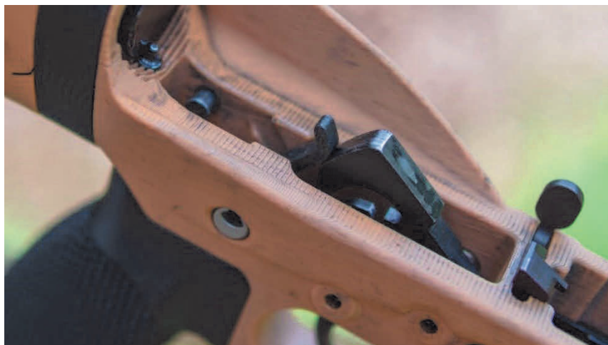
Figure 16. Super Safety installed in a lower.
